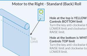
Controls BOTTOM limit Turn the key anti-clockwise to LOWER limit and clockwise to
