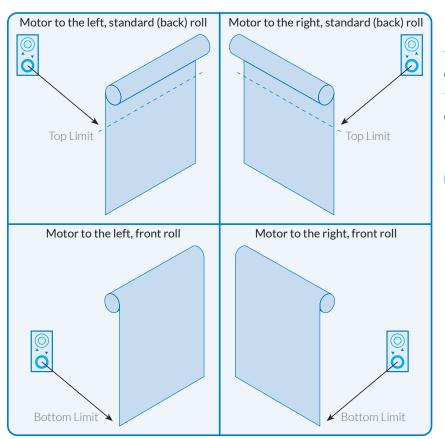
To increase the limit, turn the dial in the plus direction (ie anticlockwise)
