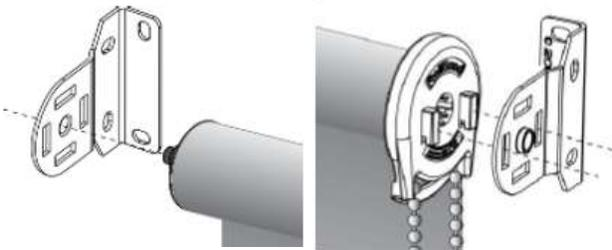
always point straight down. Attach the small plastic ball chain stopper onto the chain so that it can't be rolled past its limit.
