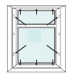
Now tighten the screws holding the frame in place.
