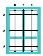
**A.** Measure the width in mm's in three places, Top, Centre and Bottom. Measure from the inside opening edge of the recess to the opposite edge. Use the smallest of the three measurements.
